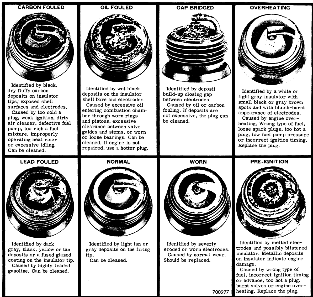
Figure 30 - Spark Plug Conditions and Causes
