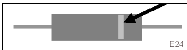
Fig. 2 Marking of the cathode
