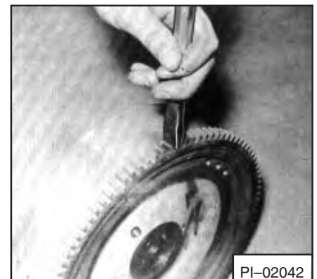
Fig. 7B-105 Removing Ring Gear
