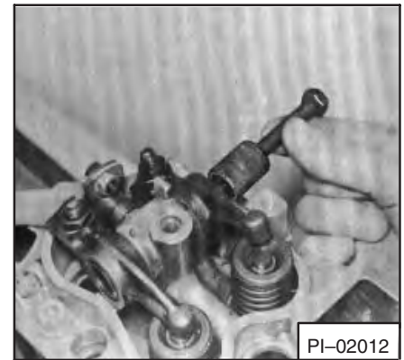
Fig. 7B-27 Removing Bushing
