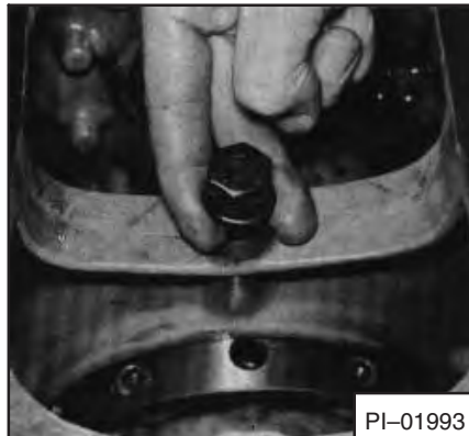
Fig. 7B-100 Installing Crankshaft
