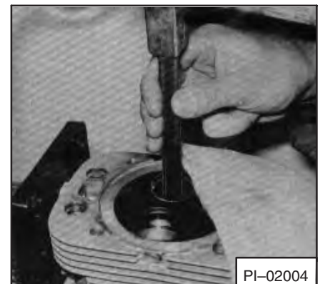
Fig. 7B-31 Removing Valve Guides
