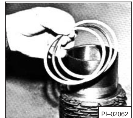
Fig. 7A-34 Installing Shims
