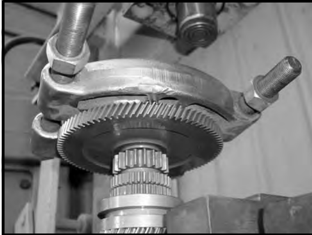
Figure 16-22 Position Large Helical Gear and Bearing
