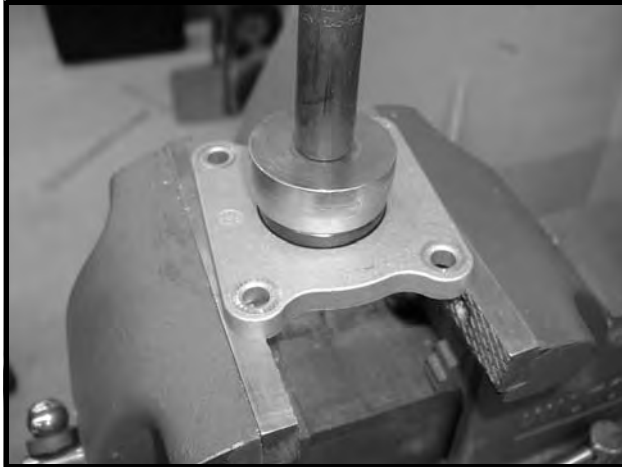
Figure 17-30 Install New Input Shaft Seal
