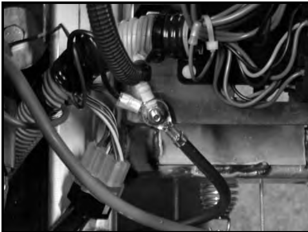
Figure 11a-6 Frame Ground
