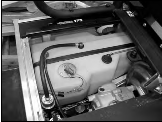
Figure 13c-13 Diesel Fuel Tank
