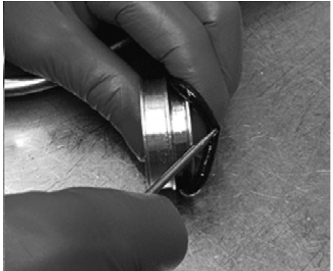
19. Pour the shock oil out of the “piggy-back” body assembly.
