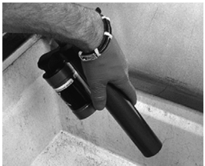
20. Using a 5/8-in. wrench, remove the LSC assembly from the eyelet, thoroughly clean the assembly, replace the O-rings, and install the assembly into the eyelet. Tighten to 14 ft-lb.
