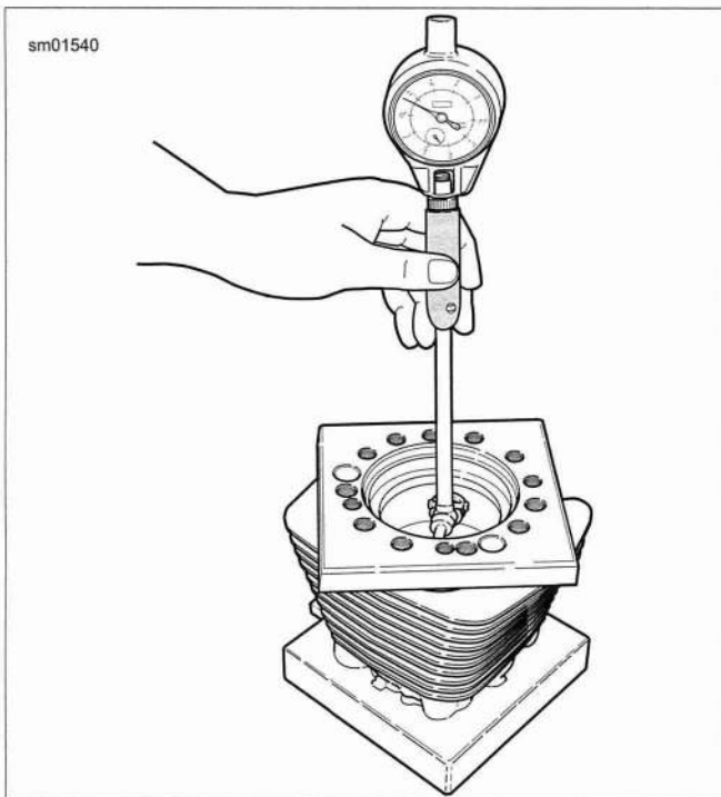
Figure 3-74. Measuring Cylinder Bore
