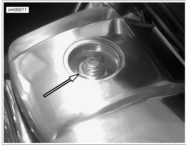
Figure 1-72. Headlamp Clamp Nut: Sportster Models
