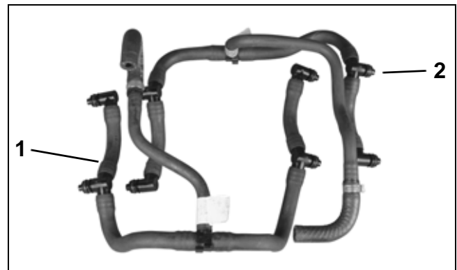
1. Fuel supply manifold 2. Fuel return manifold
