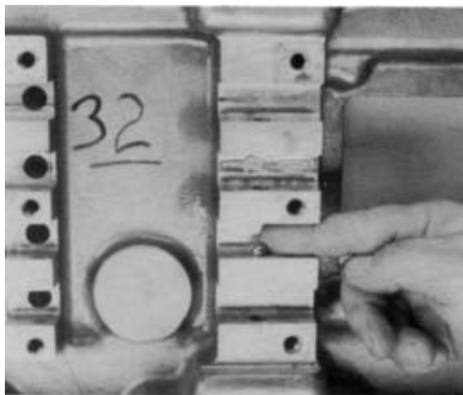
16. Install interlock balls in the shift bar housing in the following sequence: position two interlock balls in the 1st-2nd crossbore; 3rd-4th crossbore; and the 5th-6th crossbore.
