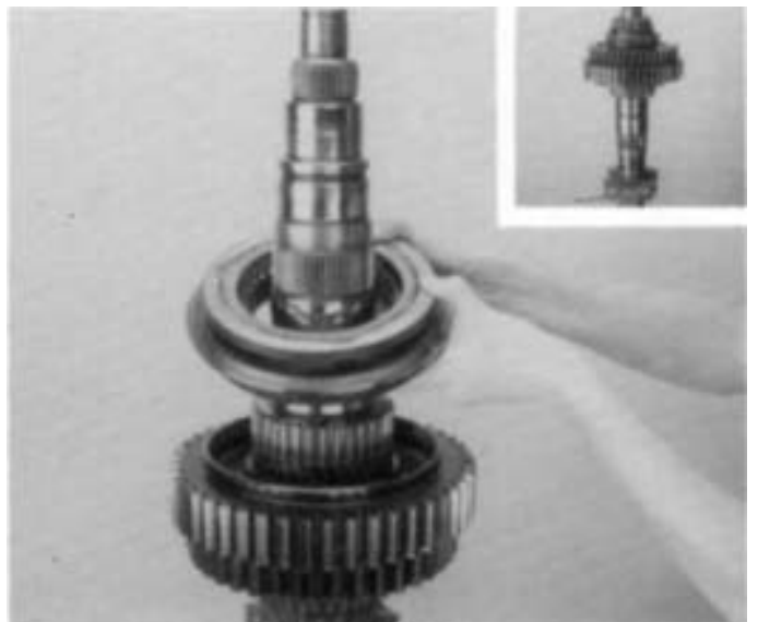
14. Remove 1st-2nd speed synchronizer assembly from the mainshaft. Reposition the mainshaft in a vise, as shown, mainshaft rear facing up (inset).
