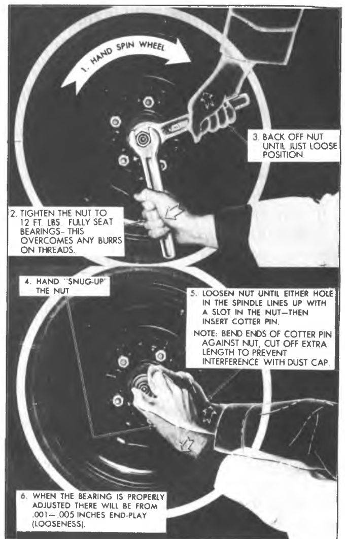
Fig. 3C-3--Wheel Bearing Adjustment
