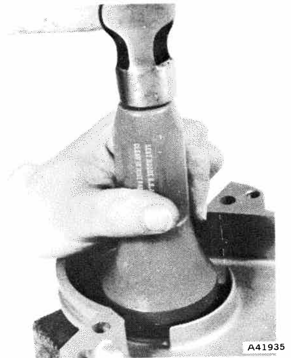
Fig. 1B-22 Timing Chain Cover Oil Seal Replacement
