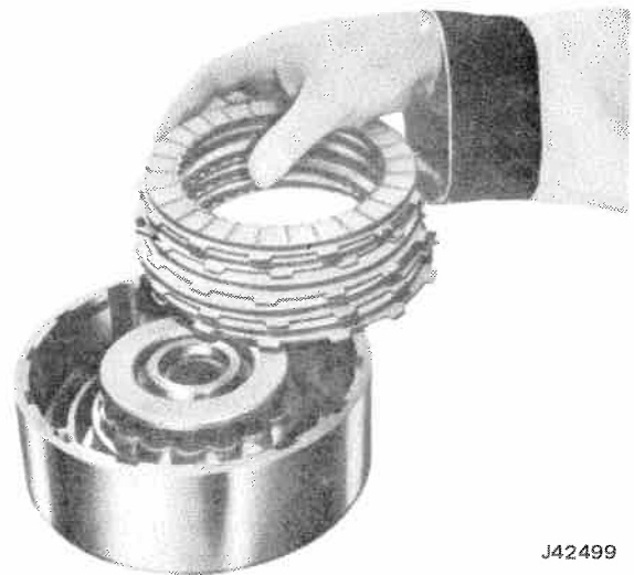
Fig. 7-69 Installing Forward Clutch Plates
