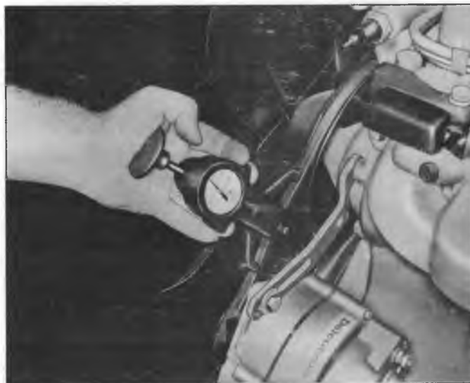
Fig. 8—Checking Belt Tension
