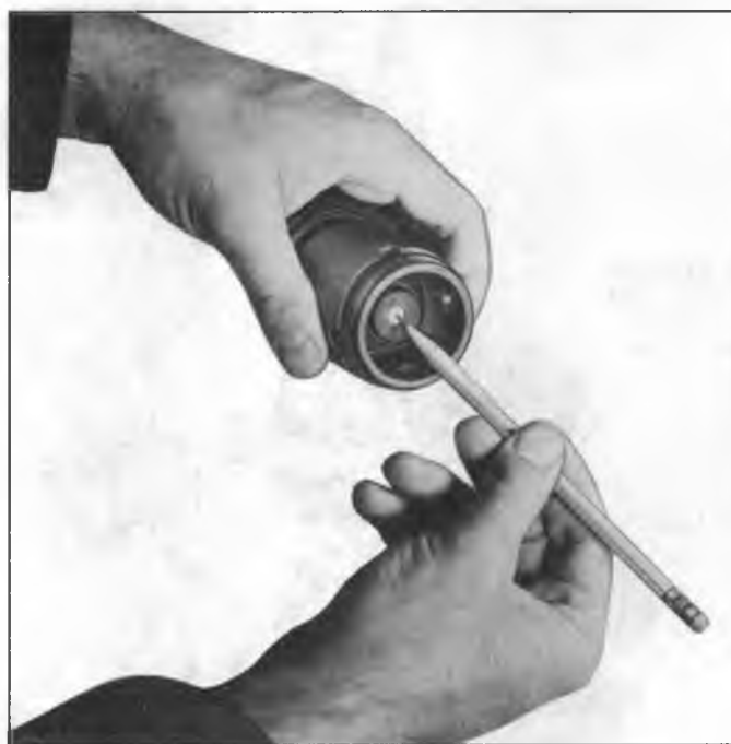
Figure 43—Removing Reaction Piston and Reaction Disc From Secondary Power Piston
