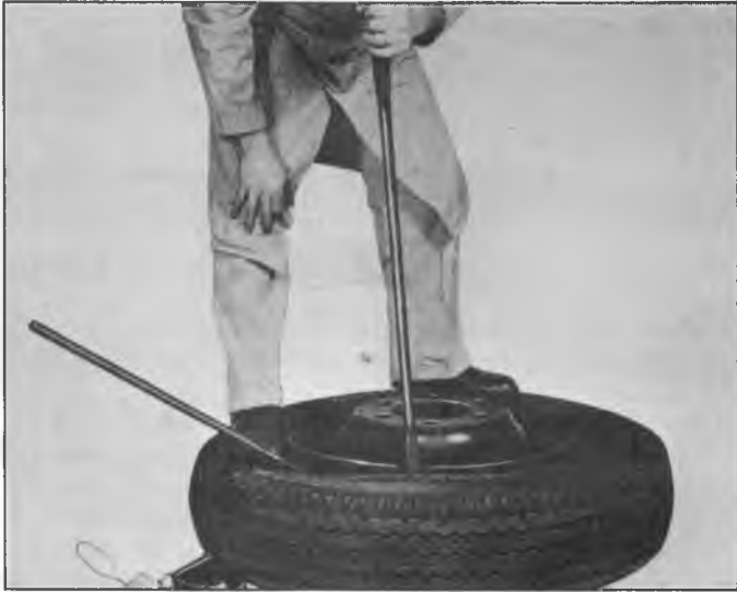
Fig. 4—Inserting Tire Iron to Lift Bead
