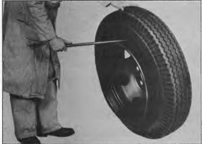
Fig. 6—Inserting Tire Iron in Second Bead
