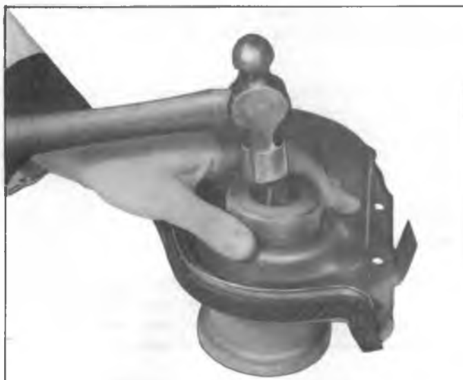
Fig. 13V—Installing Oil Seal (Cover Removed)
