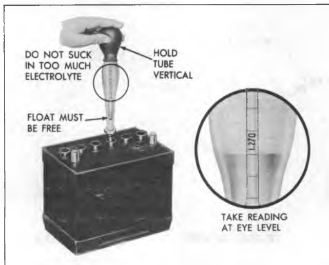
Fig. 7—Testing Specific Gravity of Battery
