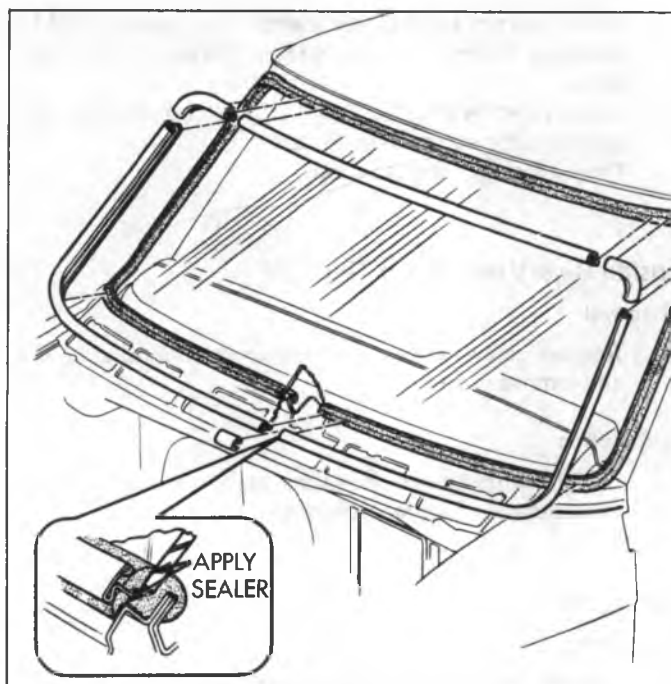
Fig. 7—Windshield Glass, Weatherstrip and Sealing
