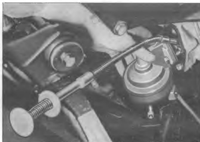
Fig. 2p—Installing V8 Engine Fuel Pump
