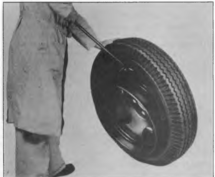
Fig. 7—Prying Second Bead from Rim
