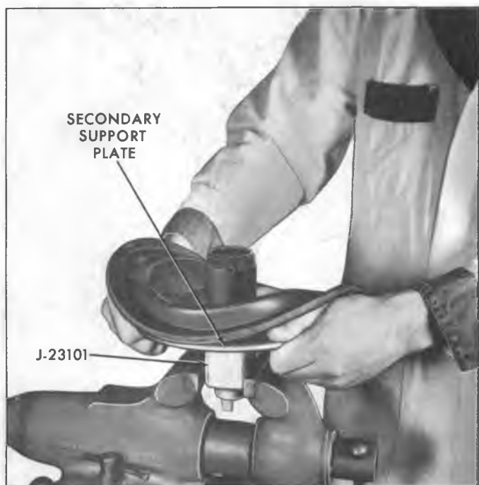
Figure 42—Locking or Unlocking Secondary Support Plate and Secondary Power Piston
