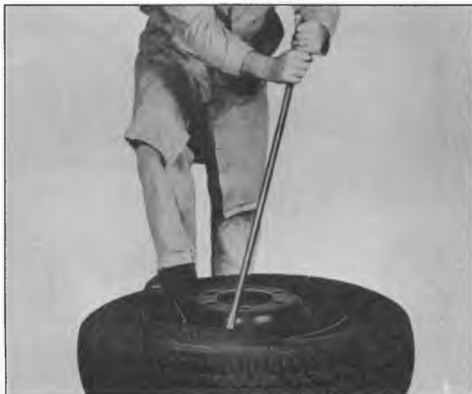
Fig. 5—Lifting Bead Over Rim
