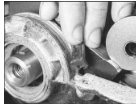
5.6b Fitting the sump gasket sealing strips to overlap the tabs on the gasket
