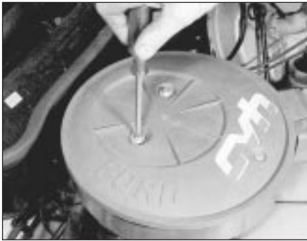
34.1a Removing the air cleaner retaining screws on a 1.3 litre CVH engine . . .
