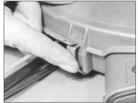
34.2 Release the air cleaner lid retaining clips, where fitted
