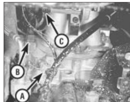
11.76 Coolant temperature sensor (A) thermo-time switch (B) and auxiliary air device (C) multi-plugs on RS Turbo models
