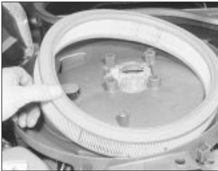
34.3 Removing the air cleaner element
