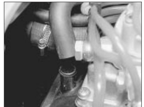
34.9 Detach the hose from the front of the air cleaner cover - K-Jetronic system
