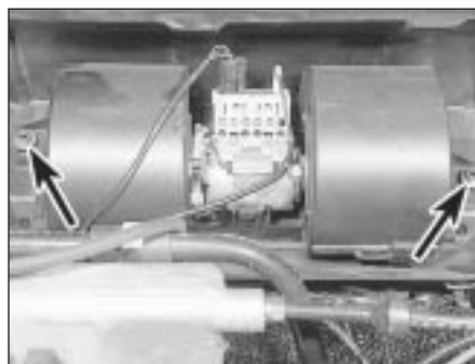
6.11 Undo the fan motor retaining nuts (arrowed)
