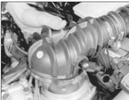
34.6b . . . and lift the air duct away from the sensor plate unit - K-Jetronic system
