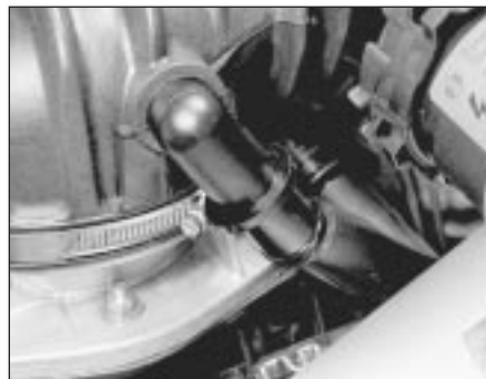
34.7 Detach the shut-off valve hose - K-Jetronic system
