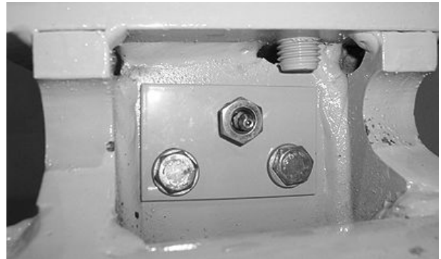
Crossbar Lubrication Line
