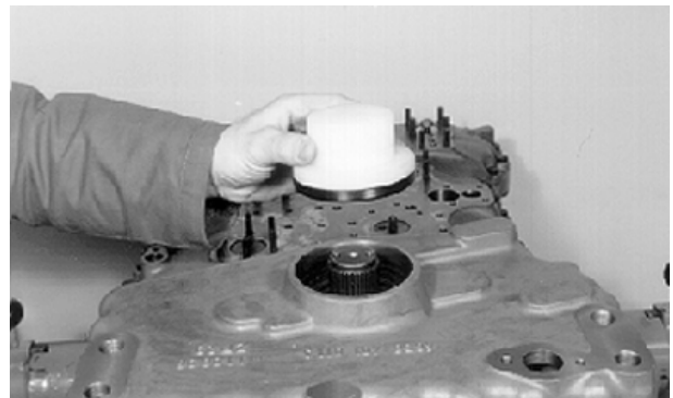
Shaft Seal Installation
