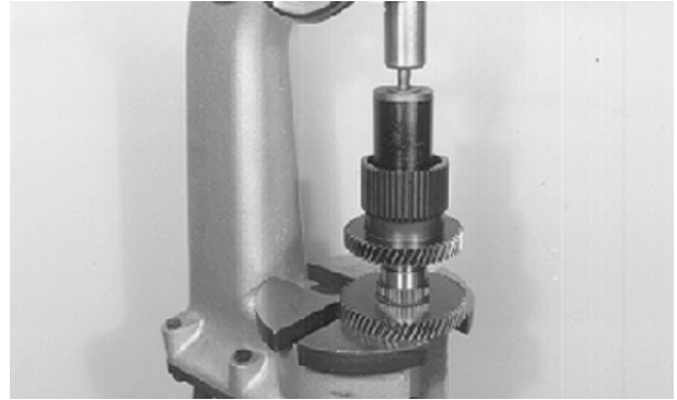
Press Idler Gear Against Shoulder
