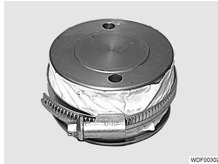
Fig. 168 Compression of the annular seal
