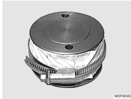
Fig. 197 Compression of the sealing ring
