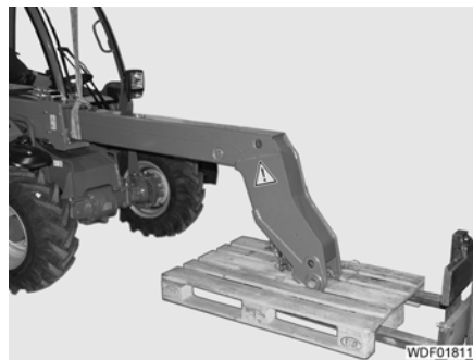
Fig. 533 Setting down the inner tube
