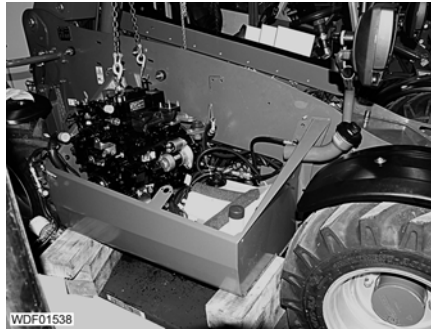
Fig. 109 Lifting out the engine
