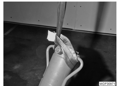
Fig. 213 Securing the tipping cylinder
