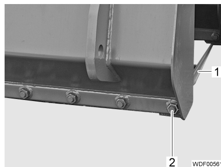
Fig. 593 Securing the prong
