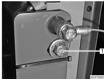
Fig. 78 Side attachment of the radiator
