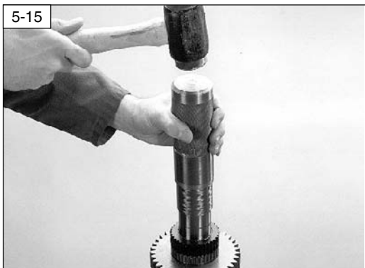
5-15 Using an appropriately sized tube refit the 1st gear bearing sleeve.
