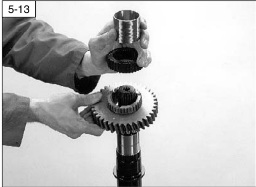
5-13 Removal of the bearing sleeve, synchro hub and 2nd gear.
