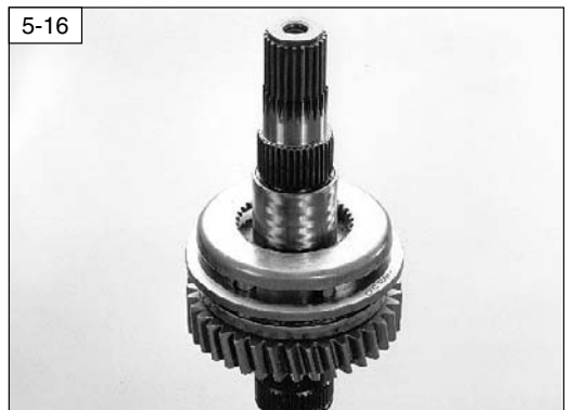
5-16 Replace the 1st / 2nd synchroniser assembly.
