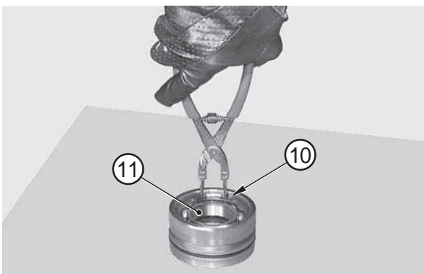
FIGURE 7: Fit the snap ring (10) on the bearing (11).
