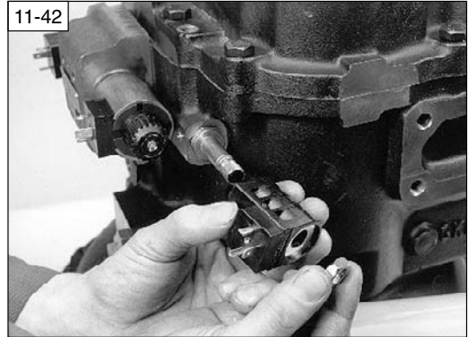
4WD VERSION : Re-fit the 4 wheel drive solenoid coil and nut. Tighten to a torque of 4 lbs / ft maximum.
