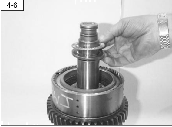
Remove the needle bearing and thrust washer.
