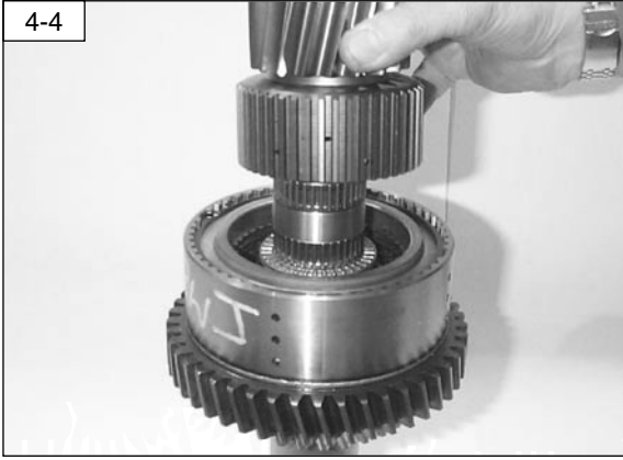
Remove the Speed Clutch 1 primary gear.
