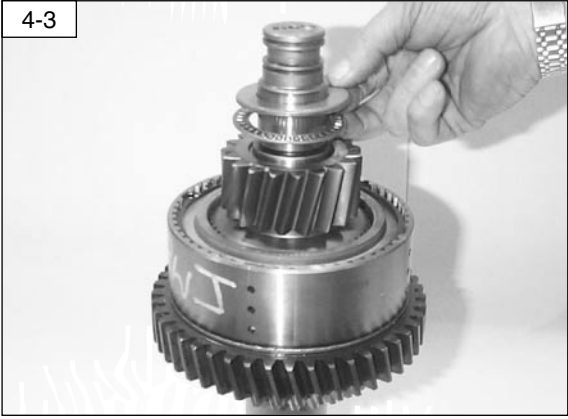
Remove the thrust washer and needle bearing.
