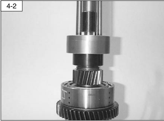
Using the appropriate bearing puller remove the rear bearing. (Tool No. 563392)
