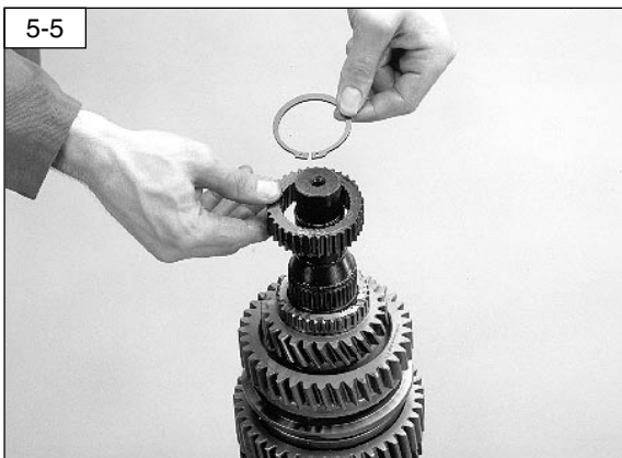
Remove the circlip and synchro hub.
