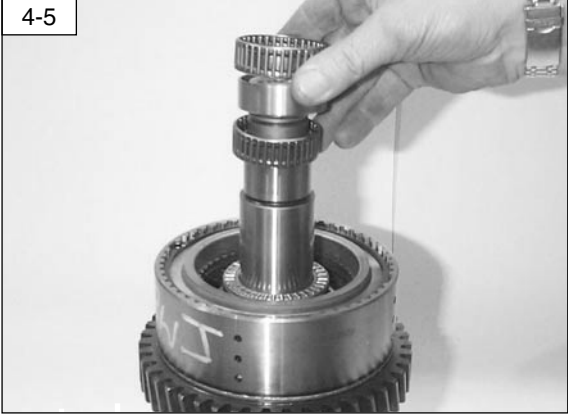
Remove the two bearings and spacer.
