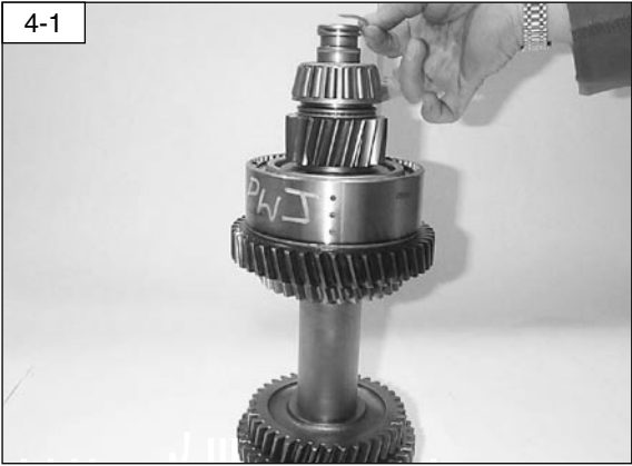
Position the shaft in a soft jawed vice as shown and remove and discard the 2 sealing rings.
