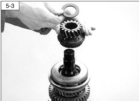
Remove the thrust washer and 4th gear.
