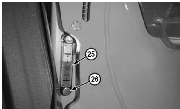
Hydraulic Oil Reservoir Sight Glass
