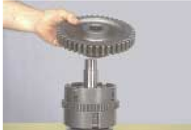
Figure 208 Install the clutch gear in the clutch assembly by aligning the clutch hub teeth with the clutch inner discs. Make sure the clutch hub is fully engaged in the clutch assembly. Do not force this operation.
