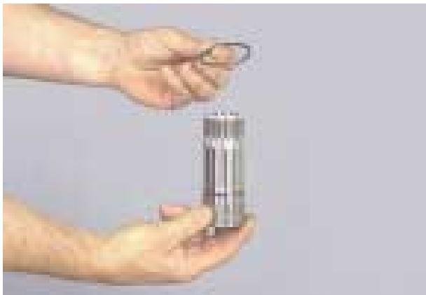
Figure 326 Install oil sealing ring on expander ring. NOTE: Expander spring gap is to be 180° from sealing ring hook joint.
