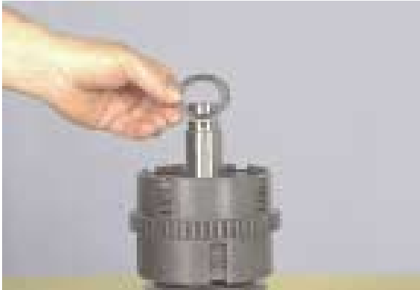
Figure 205 Position thrust bearing on clutch shaft against inner thrust bearing washer.
