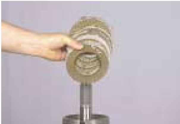
Figure 85 Remove inner and outer clutch discs.
