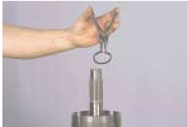
Figure 88 Remove retainer ring retainer.
