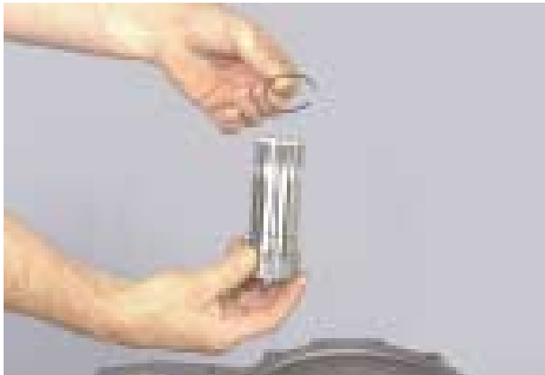
Figure 325 Install stator support oil sealing ring expander ring.
