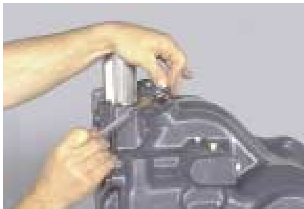
Figure 385 Install sensor hole plug and O-ring.
