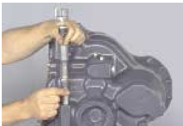
Figure 387 Install dipstick tube and dipstick.
