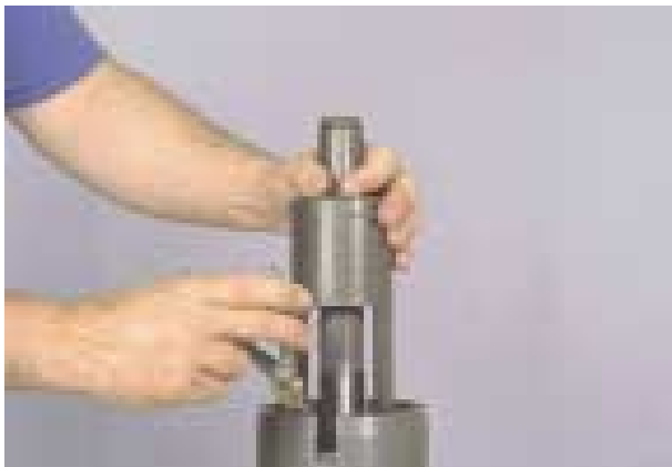
Figure 86 Compress disc springs and remove retainer ring.
