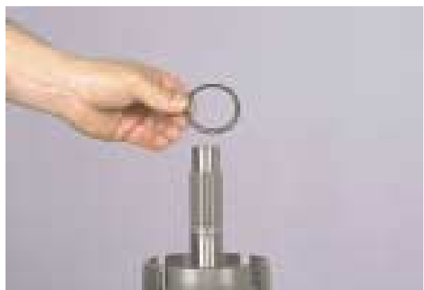
Figure 90 Remove clutch piston wear plate.
