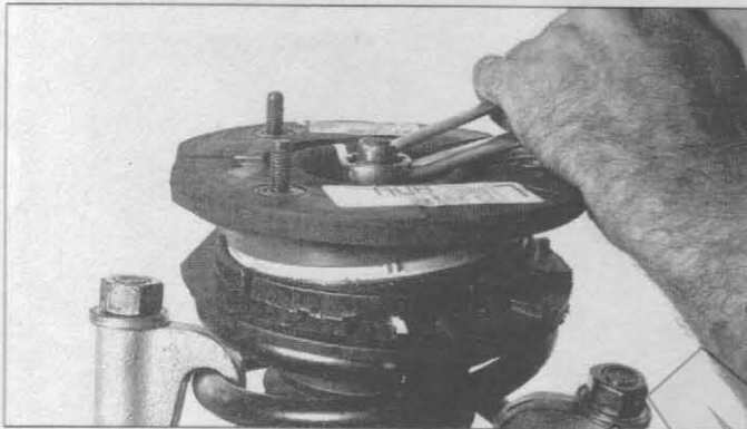
4.5 Using a wrench on the damper shaft to prevent it from turning, loosen the damper shaft nut
