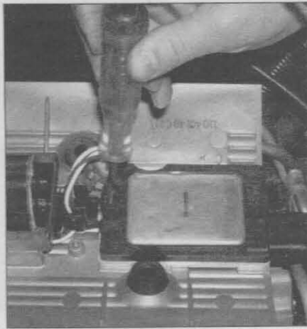
6.16b ... then connect an LED test light to the positive terminal of the battery and to each of the coil negative (-) terminals on the ignition module and watch for a blinking light when the engine is cranked
