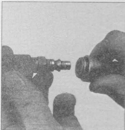
6.4 This is what the air hose adapter that threads into the spark plug looks like - they're commonly available from auto part stores
