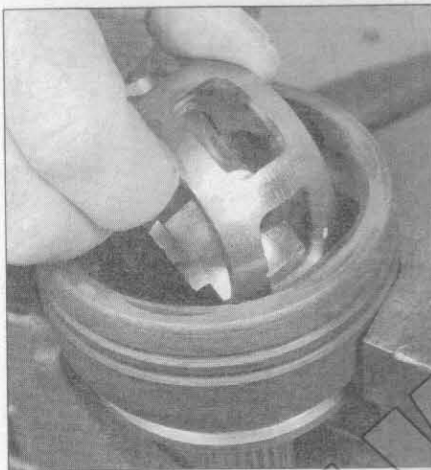
11.4l With the race and cage tilted at 90-degrees, lower the assembly into the housing
