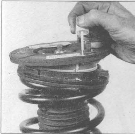
4.3a Mark the relationship of the coil spring to the upper spring seat and insulator and to the strut mount...
