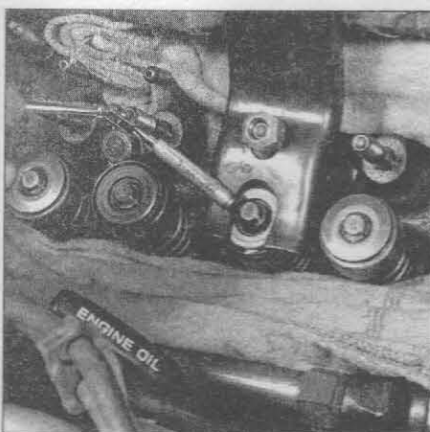
6.9 Once the spring is depressed, the keepers can be removed with a small magnet or needle-nose pliers (a magnet is preferred to prevent dropping the keepers)
