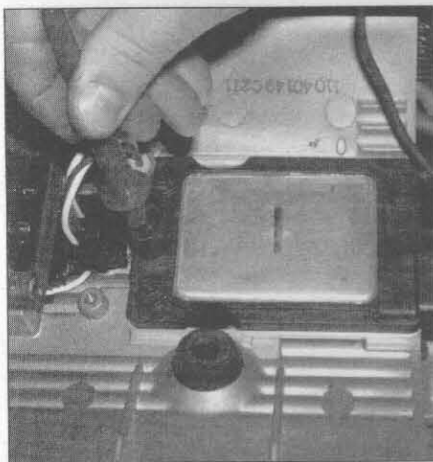
6.16a On 2.3L and 2.4L engines, first disconnect the ignition coil-to-ignition module connector and check for battery voltage to the coil with the ignition key On ...
