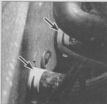
11.3 Disconnect the heater core hoses (arrows) at the engine compartment firewall
