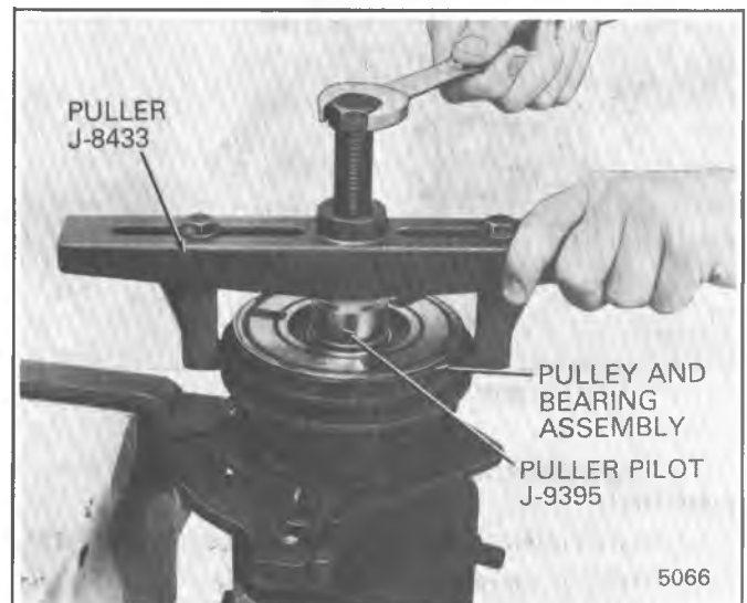
Fig. 1D-10 Removing A-6 Pulley and Bearing Asm.
