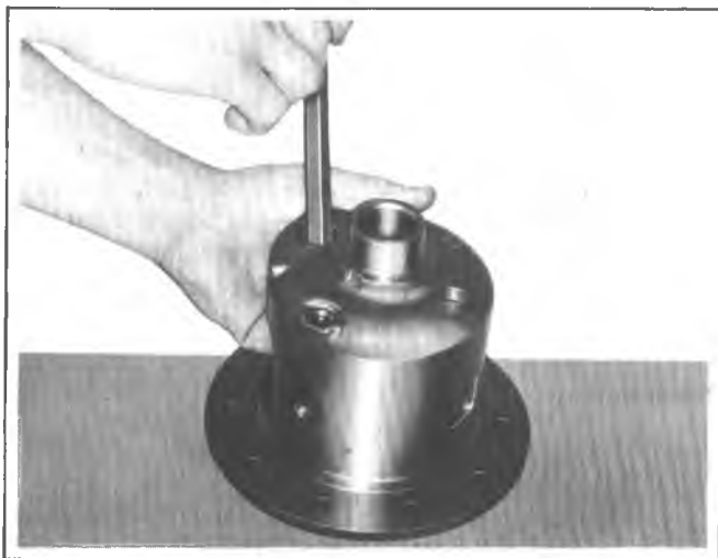
Fig. 8D--Removing Side Gear
