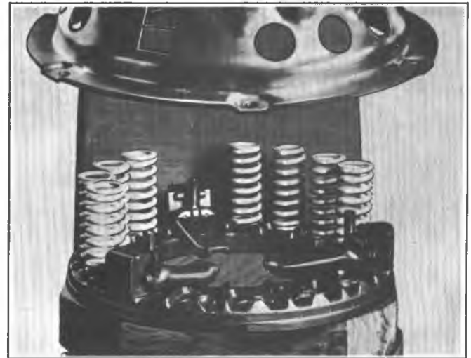
Fig. 7C-10E-Assembling Cover and Pressure Plate
