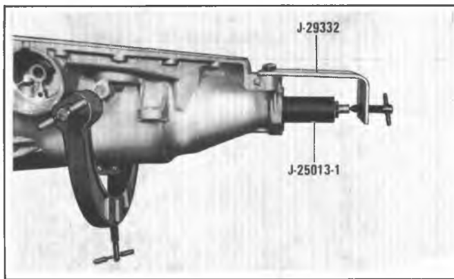
Figure 7A6-32 Installing Tools on Rear End of Case
