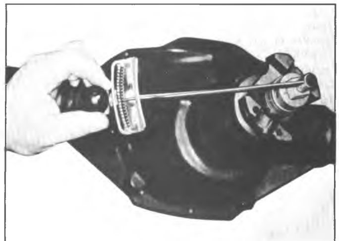
Fig. 26B--Measuring Rotating Torque
