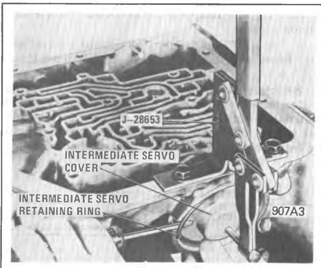
Figure 7A1-19 Removing Intermediate Servo Retaining Ring
