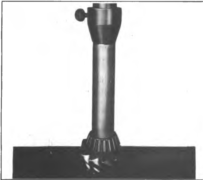
Fig. 24B--Installing Rear Bearing
