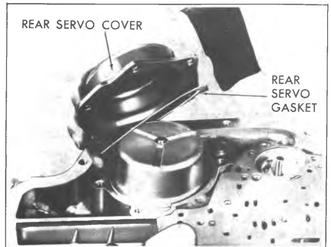
Fig. 7A-182C--Installing Rear Servo Cover and Gasket
