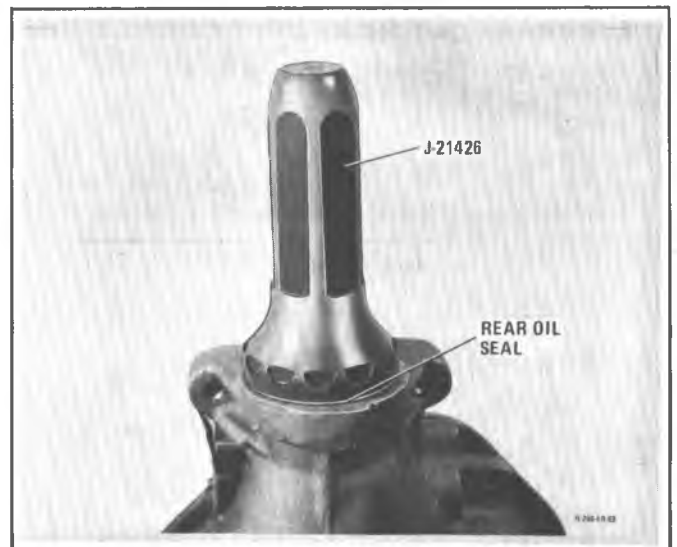
Figure 7A6-81 Installing Rear Oil Seal
