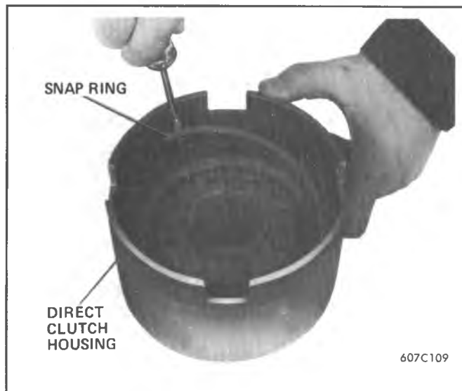
Figure 7A1-110 Removing Direct Clutch Snap Ring
