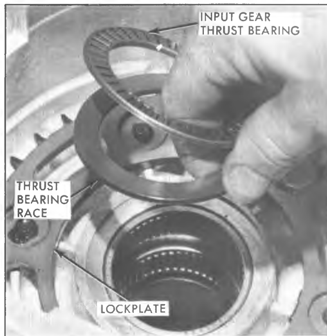
Fig. 7E-16-Input Gear Thrust Bearing and Race Removal&Installation
