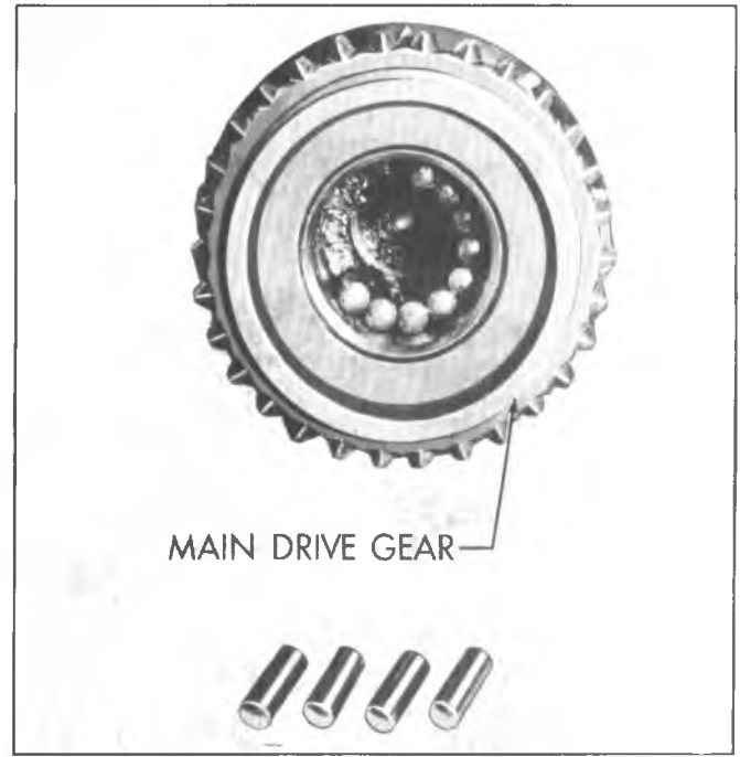
Fig. 7B-20J--Loading Mainshaft Bearings
