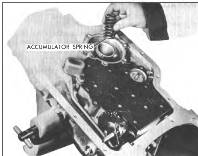
Fig. 7A-180C--Installing Rear Accumulator Spring
