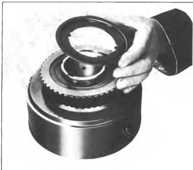
Fig. 7A-109C--Installing Intermediate Clutch Retainer
