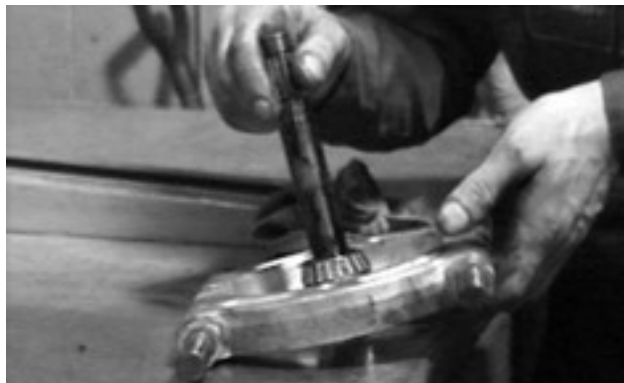
Figure 7-38. Lower Pinion Bearing Removal
