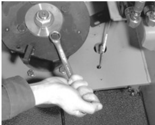
Figure 7-9. Removing Steering Plate Bolts
