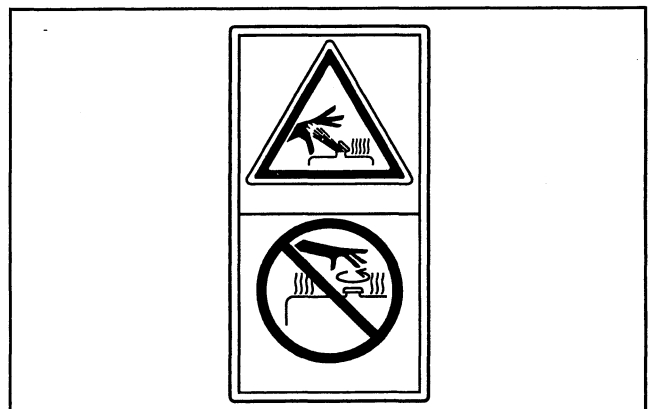
RELEASE HYDRAULIC TANK PRESSURE
