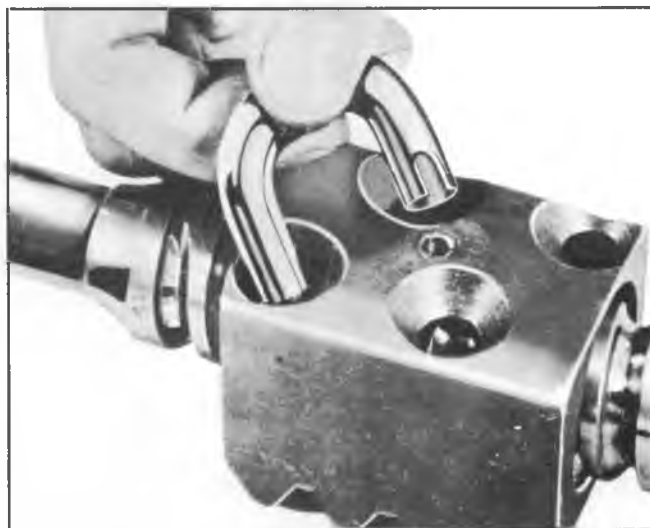
Fig. 13--Removing and Replacing Ball Guide
