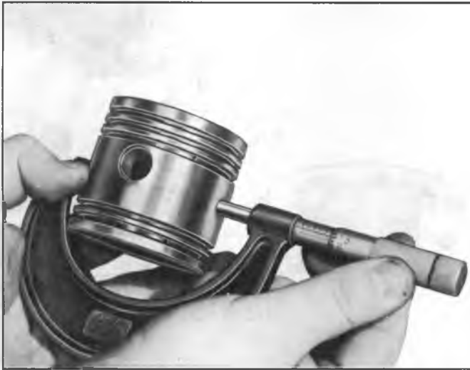
Fig. 10G--Measuring Piston Diameter
