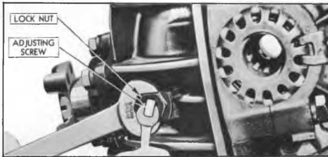
Fig. 19G—Ring Gear Thrust Pad Adjustment
