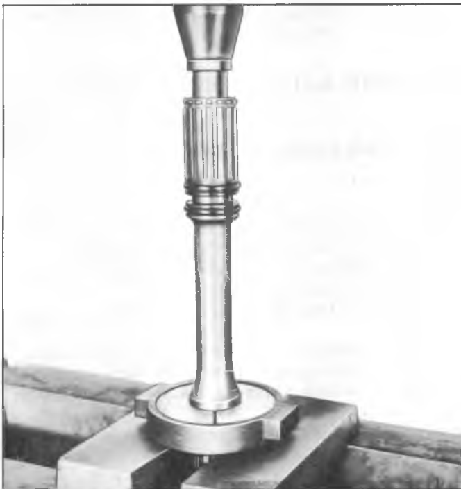
Fig. 21M—Installing Output Shaft Bushing Using Tool J-8476
