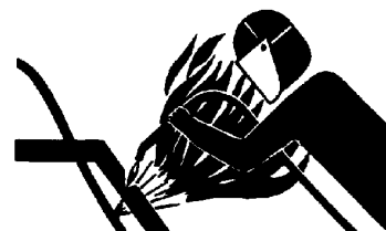
Heating Near Pressurized Fluid Lines
