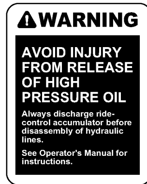
WARNING, Avoid Injury From Release of High Pressure Oil
