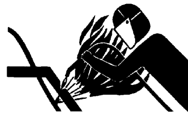
Heating Near Pressurized Fluid Lines
