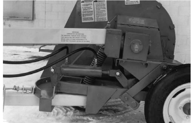
Fig. 48: Optional Hydraulic Lift & Cylinder Kits (Installed)
