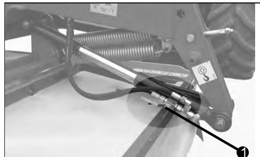
Fig. 62 Ball valve on the left lifting cylinder open
