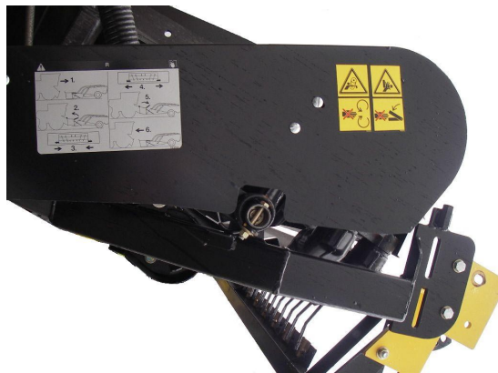
Rotating Drive Hazard, Pinch Point Located on Belt Guard
