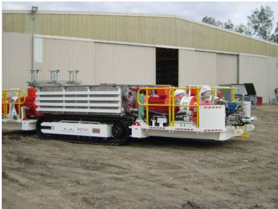
Pump station and crawler unit
