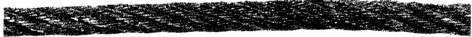
Figure 59. This rope was subjected to repeated bending over sheaves while under normal loads. Fatigue breaks in the individual outer wires resulted. The wire breaks are square-end and the majority are found on the crown of the strands.
