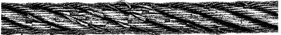
Figure 61. A typical example of localized wear. The cumulative effect can be minimized and the rope life extended if a suitable cut-off practice was employed.
