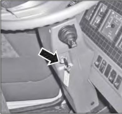
Steering lock cum ignition key
