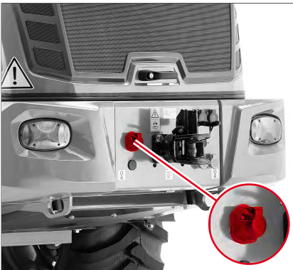
Fig. 145: 7-pole plug receptacle at the rear
