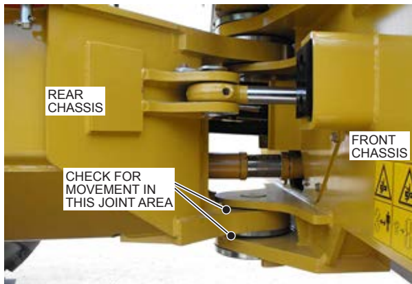
620E-066 CENTRE JOINT PRE-LOAD CHECK
