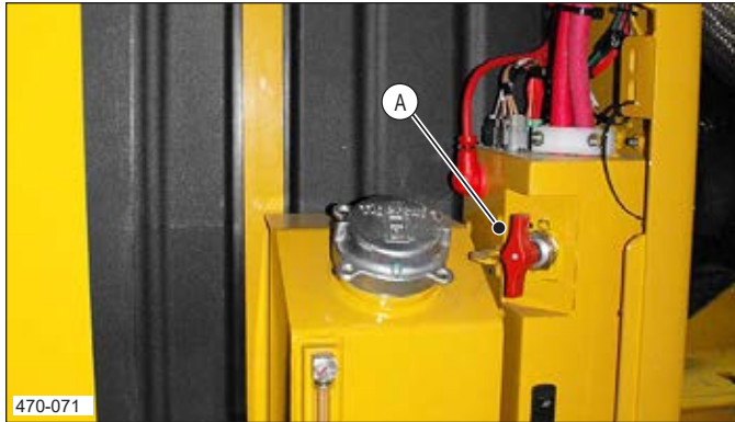
A Battery Disconnect Switch (Right Rear Storage Compartment)
