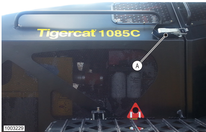
A Engine Hood Latch, Later Design
