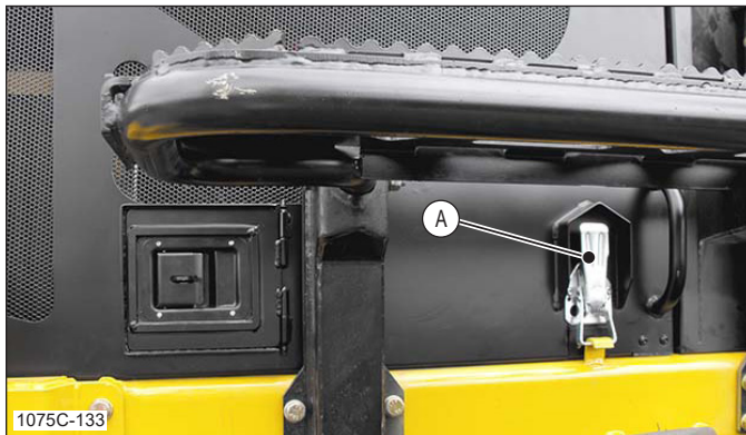
A Engine Hood Latch, Earlier Design
