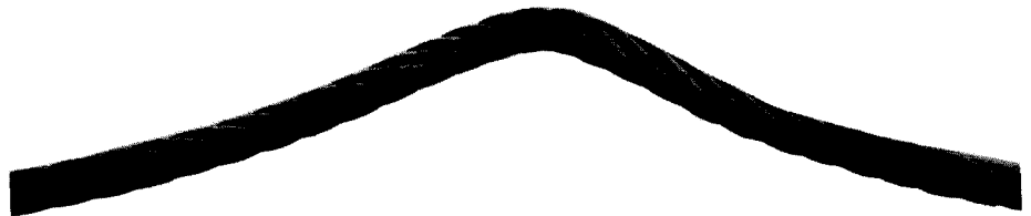
Figure 47. This rope condition is called a dog leg .
