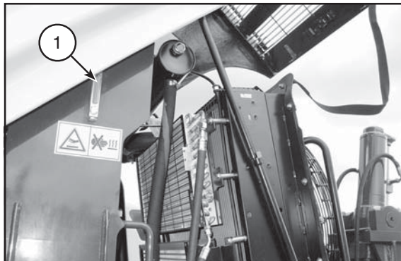
1. HYDRAULIC OIL LEVEL GAUGE
