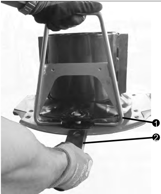
Fig. 92 Removing the cutter blades
