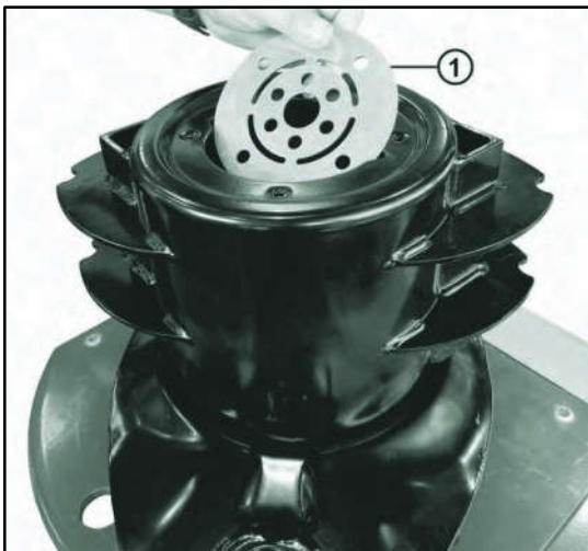
Fig. 71 Insert new driveGUARD element
