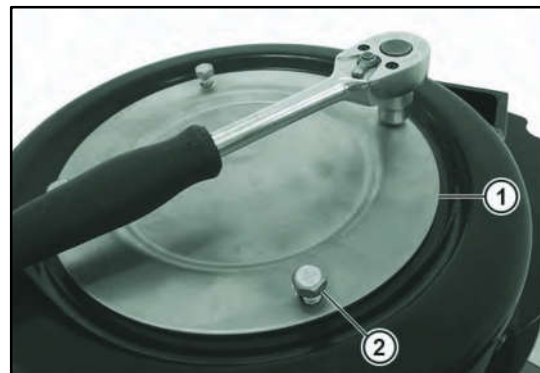
Fig. 74 Bolt down cover
