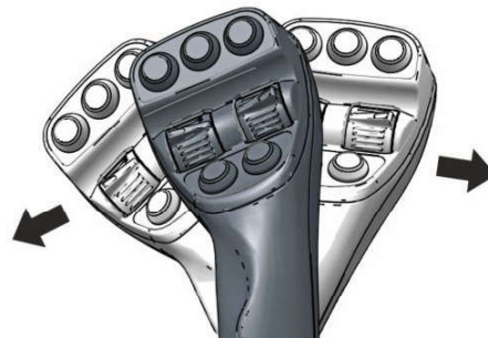
Fig. 331: Activating the shake/vibrate function
