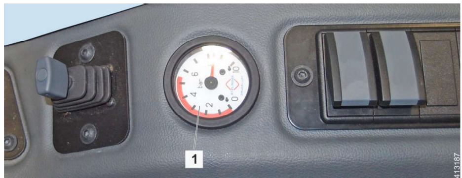
Fig. 357: Air brake system pressure gauge
