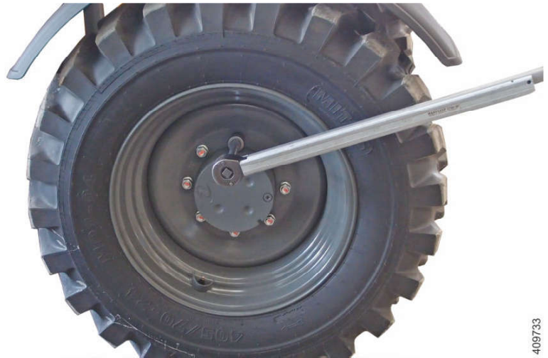
Fig. 537: Check the wheel lugs
