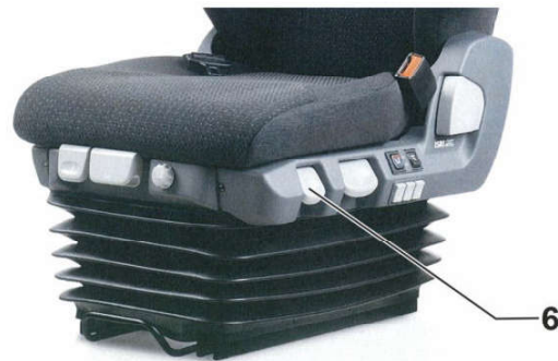
Fig. 209: Adjusting the shock absorber
