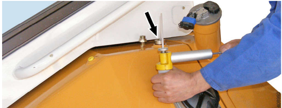
Fig. 425: Oil sampling location - hydraulic system
