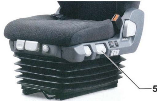
Fig. 208: Adjusting the horizontal suspension
