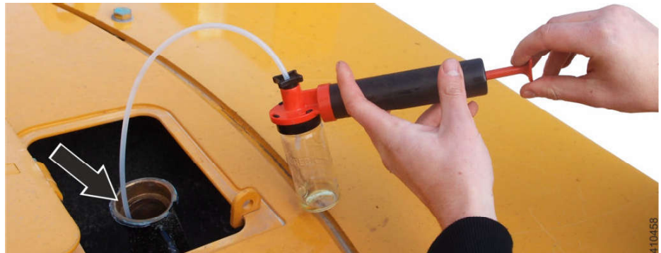
Fig. 426: Coolant oil sampling location
