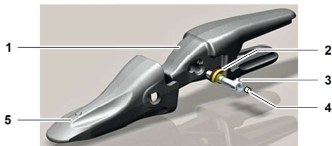
Fig. 633: Changing bucket teeth with Z system
