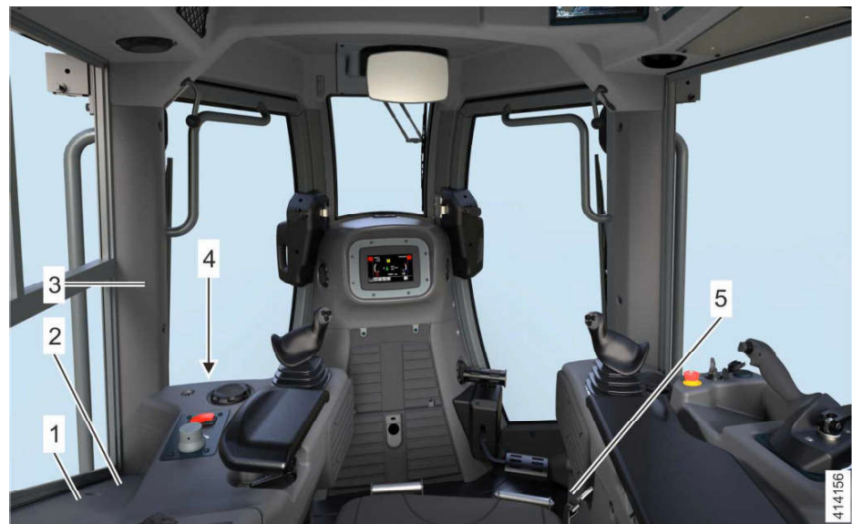
Fig. 29: Location of safety signs in the operator's cab
