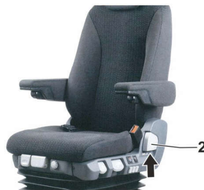
Fig. 341: Adjusting the backrest incline
