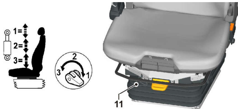
Fig. 322: Adjusting the shock absorber
