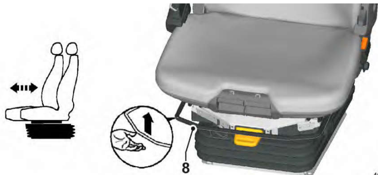
Fig. 189: Adjusting the operator's seat horizontally
