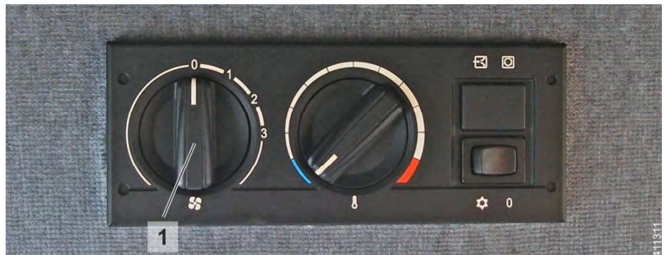
Fig. 226: Rotary switches for blower
