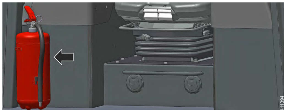
Fig. 244: Mounting location of fire extinguisher
