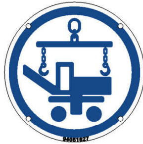
Fig. 72: Lifting point sign
