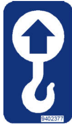
Fig. 71: Lifting point sign
